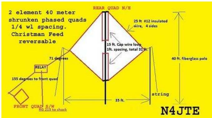
How do you shrink 2 full size quads without killing the gain and bandwidth? Is there any way an almost ground mounted diamond shaped quad array will do anything?
