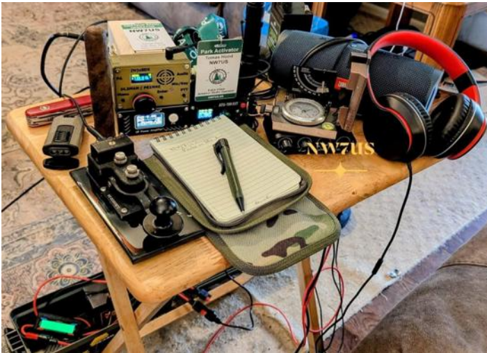
My POTA / Portable HF station (a low-power, or, QRP, station).
