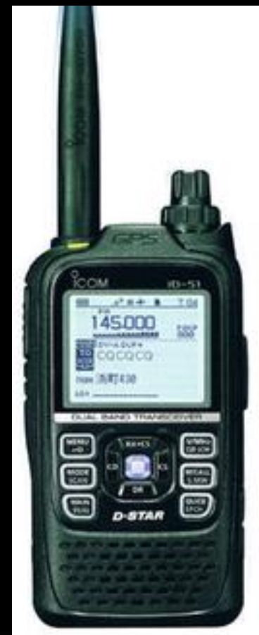
Icom ID-51 Plus 2m/70cm Internal GPS Faster DV transfer RS-MS1A Android Application DV/FM repeater search
