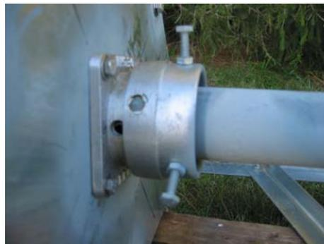
*Second thrust bearing detail. Note the hole drilled through the side near the base for a pin in case the rotator has to be removed for service.*
