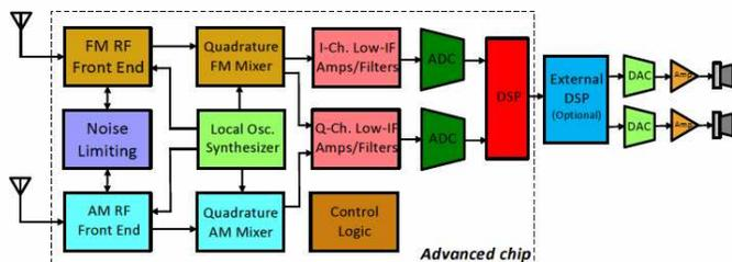
Figure 8 - Typical Advanced Receiver Architecture
