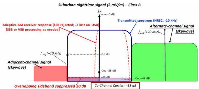
**Figure 6 - Receiver Fringe Frequency Response**
