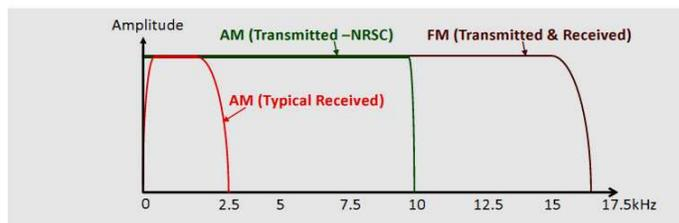
Figure 1 – FM Vs. AM Audio Frequency Response
