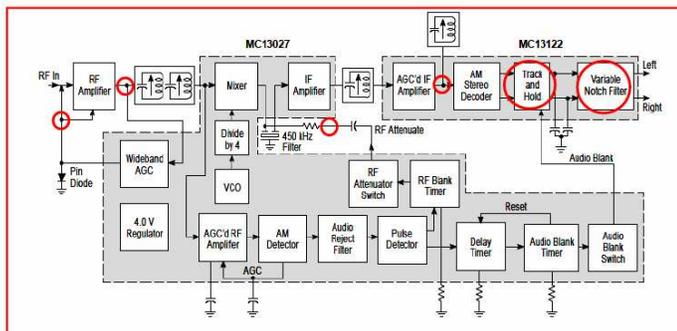
Figure 2 – Motorola AM Receiver With Advanced Noise Limiting
