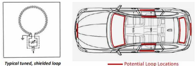
Figure 9 - Vehicle H-Field Implementations
