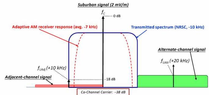
**Figure 5 - Receiver Suburban Frequency Response**
