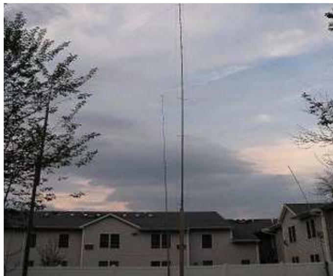
Long story short, a little pruning got me to 7.150 on both. I hooked up the previous phaselines to the outside corners and checked at the radio. I got a 1.7 swr in each direction, workable with no tuner required.
