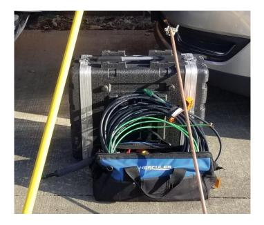
This Go-Kit was first unveiled at the 2021 Field Day held on the Collins Aerospace campus. It consists of an ICOM IC-7300 as the XCVR with a switching power supply. There's a number of ancillary devices which enhance the utilization of the Kit. In addition, it includes an 80-10M EFHV antenna, ground rod and antenna support pole. Come to the meeting to learn more about the Go-Kit, and, perhaps pick up some great ideas for your own kit.
